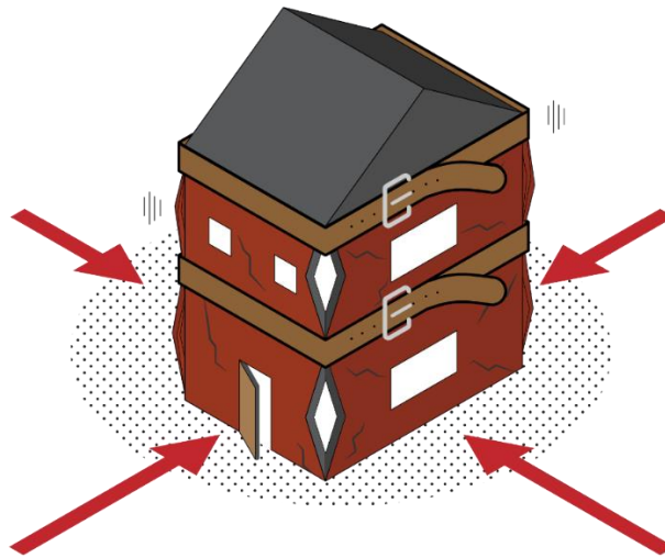
Figure 1. A damaged building during an earthquake can be held together at floor and roof level by tie or ring beams which function like strong belts.
