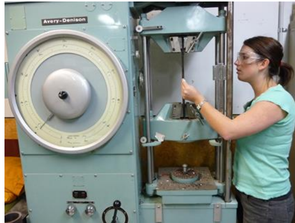
Figure 1. A reinforcing bar is being tested to check it is up to standard.
