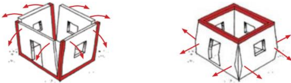
Figure 3. Walls of a simple building are not prevented from falling by columns alone. Roof-level ring or tie beams can tie the building together. (From Guide book for building earthquake resistant houses in confined masonry (World Housing Encyclopedia, 2018).
